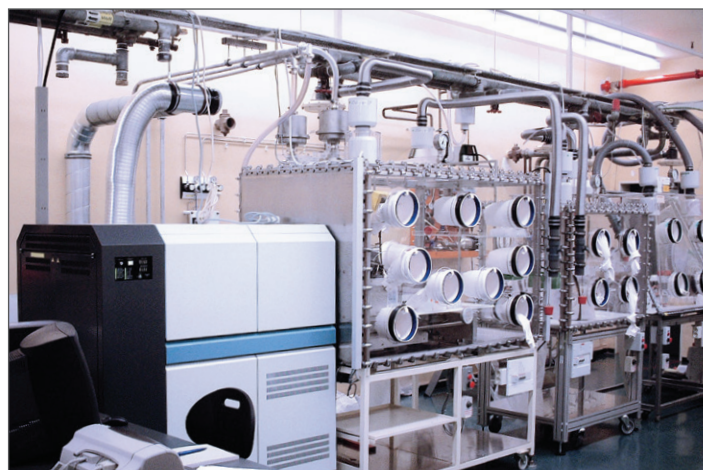
Figure 4: Element 2 ICP-MS with glove box adaption
